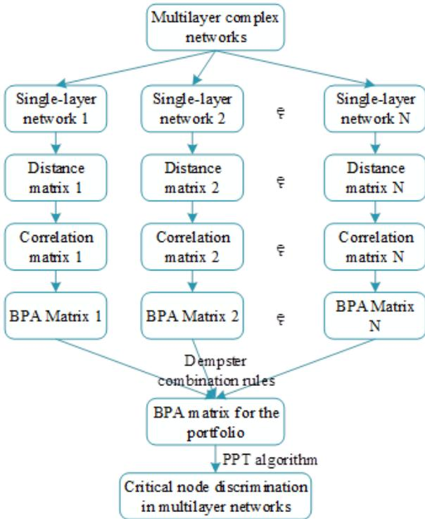
Figure 6: System evaluation model for multi-layer network
