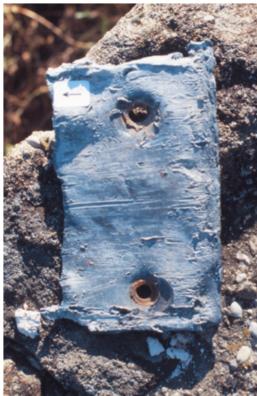
Figure 3: The lead plate as it appeared when it was removed, after 7 years on the limestone. The streaks are clearly visible. At the top right, the arrow, 1 cm long, gives the direction of snow creep.
